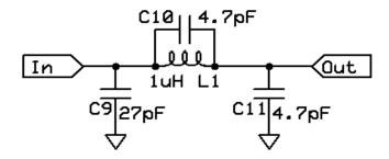
This circuit is on the PCB under each DDS Module, but the components are not included in the kit. I should note that the is also quite a bit more attenuation, so the signal is clean, but low level.
