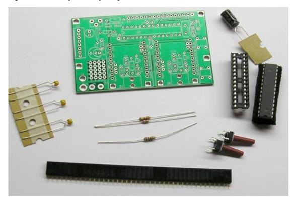
Kit as normally shipped, the female header is 40 pins, so you will need to cut it into 10, 10 and 16 pins. Some kits may ship with the connecter already cut. To cut the 40 pin one, pull out the 11th pin, then cut there. do that again for another 10 pin connector. That will leave 18 pins left, just pull out two on then end, and cut that off
