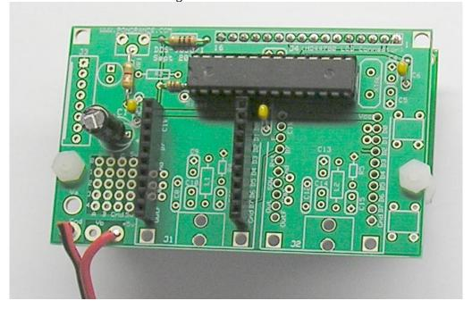
VR1 is used for LCD contrast. With the kit I ship a 3.3K fixed resistor which is soldered in as shown in the above photo. This works fine as long as the Vcc is close to 5.0 volts, with most (but not all) LCD's. If your
